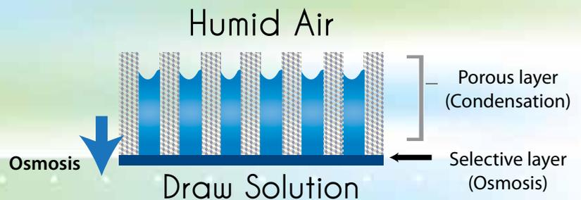
**Figure 1** - Osmotic dehydration across an anisotropic membrane consisting of a selective layer that is supported by a porous layer. Capillary condensation allows for osmosis to occur across the selective layer of the membrane into a concentrated salt or osmotic solution.
